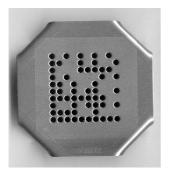
Material Size Bar code Finishing Color Temperature range Marking method Fastening 1.4301, 1.4404, 1.4435 and more As per specification Datamatrix ECC-200 Single plates None Up to 1'000°C Punching, etching Welding, screws, rivets, cable binders, inserting, etc.
